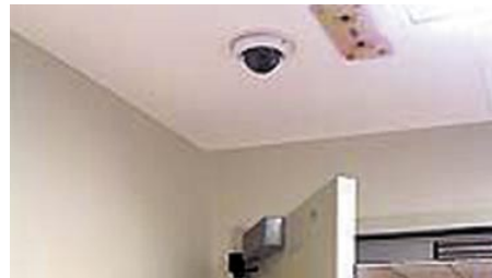
T-DAR DS100 camera in the ceiling above a corridor with a single in-swinging door.
