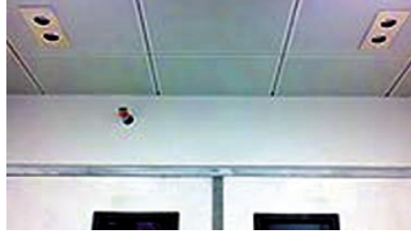
Two T-DAR DS200 cameras mounted above a double door in a standard suspended ceiling.
